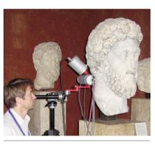
Figure 1. Portable X-ray fluorescence system and sculptures Ma1163 and Ma5101 of dolomitic marble presumably from Thasos.
