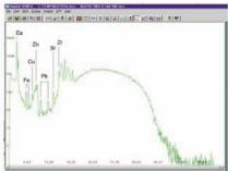
Figure 2. X-ray spectra of major elements (Mg, Ca) and trace elements (Fe, Cu, Zn, Sr, Pb).
